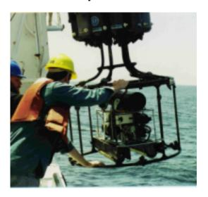
reading stored operating parameters from an EEPROM inside the CPU chip. Since CAST MODE has been selected, the CPU also measures the output of the depth sensor and saves this value as a zero-depth offset. This offset is used to correct depth values once TAPS is put into the water.
