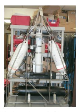
It is almost always preferable to mount TAPS to the platform with clamps (hoseclamps are suitable) around the pressure case and to use the tabs to limit fore-and-aft motion and as mounts for safety lines.
