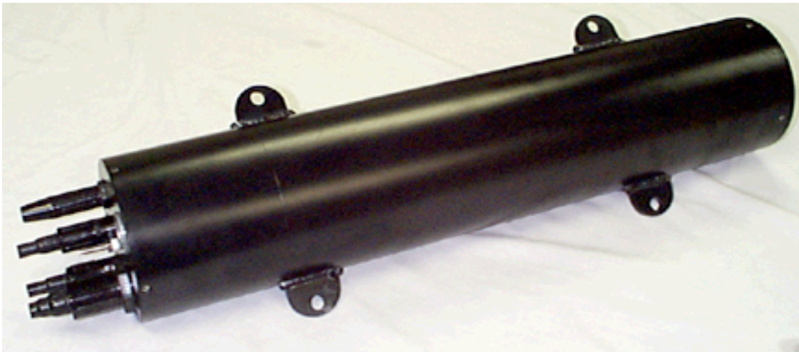
Figure 1. TAPS external views. The six acoustic transducers are the circles on the endcap visible in the top picture. Each channel uses a separate transducer. The connectors for I/O, power switching, and external sensors are visible in the lower picture, as is the thermistor. The depth sensor is on this endcap as well.
