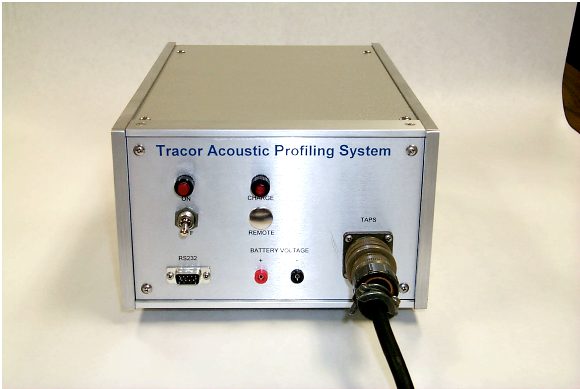
Figure 4. TAPS charger/IO unit. A TAPS interconnect cable is attached. A DB-9 connector (lower left on front panel) is supplied for connection to the serial port of a host computer. Charging voltage may be measured on the front panel test jacks. AC power and charge state are indicated on the panel lights.
