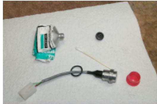
Also, clean the cavity in the endcap with cotton swabs and alcohol to remove any old grease from the machined surfaces where the o-ring seals.
