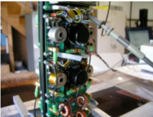
Each transmitter card contains two transmitters and two T/R switches. The frequency for each channel should be labeled on the transformer can (silver can in the figure). There are jumpers on each side near the SMA connector that leads to the tuning boards. They are not symmetric but there is only one jumper on each side in this general area. Slide the shorting plug over the appropriate jumper to enable signals to reach the receiver.
