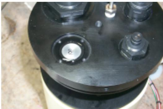
Place the neoprene cover gently in place, aligning the holes in the cover with the screw holes before dropping it into place. Lay the retaining ring in place over the cover. Install the four screws loosely, using a small dab of antiseize on each first. When all screws are installed, tighten them in rotation, a bit at a time, until all screws are snug. No particularly high torque is required to retain this assembly so be prudent.
