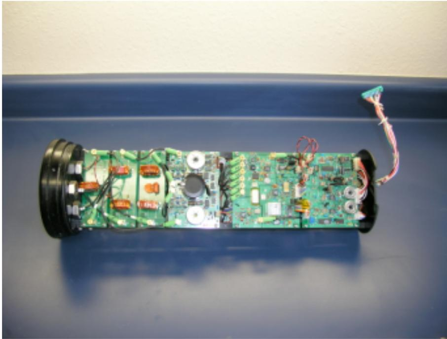
TAPS electronics assembly. Cards are fastened to an aluminum frame with screws and nylon standoffs.
