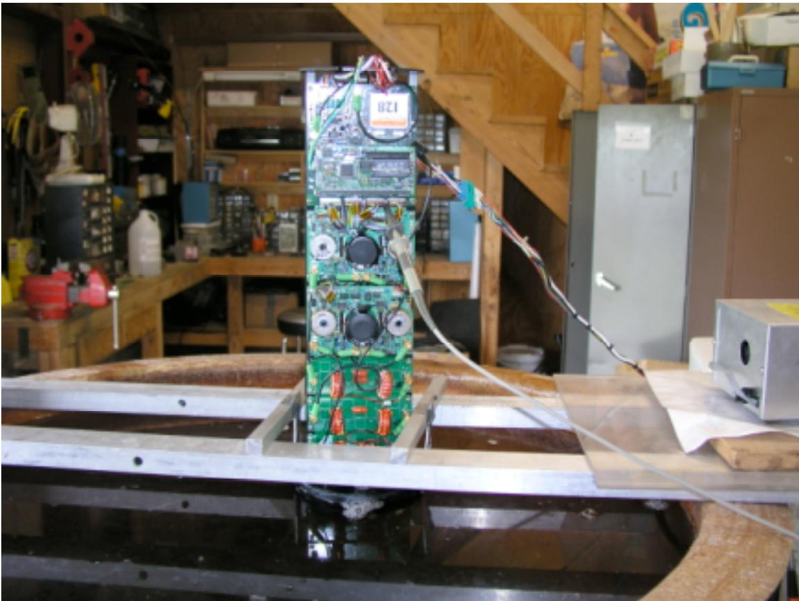
TAPS mounted on a cylindrical test tank. The horizontal tubes provide a level surface for the T-mounts to slide on when locating TAPS above the test transducers. The test transducers, in this case, are mounted on a frame on the bottom of the tank.
