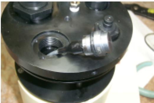
Prepare the new sensor for installation by installing an o-ring as shown below. Use a modest amount of o-ring grease on
