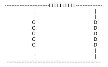
where a series inductor and parallel capacitor have been assumed.
