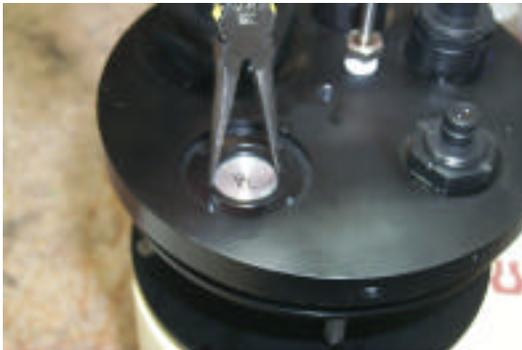
Next, disconnect the molex connector under the endcap to free the depth sensor cable and remove the depth sensor.
