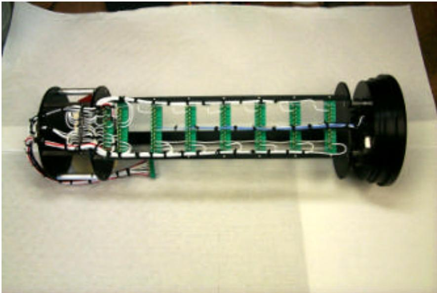
Electronics/Transducer Assembly (ETA) viewed from the wiring side. The CPU/IO card is contained in the small bay to the left. All other cards reside in the large card bay. The Power Control card is towards the left, channel 6 (3 MHz) transceiver is towards the right. The black bar visible behind the connectors is the PCB retainer strap.
