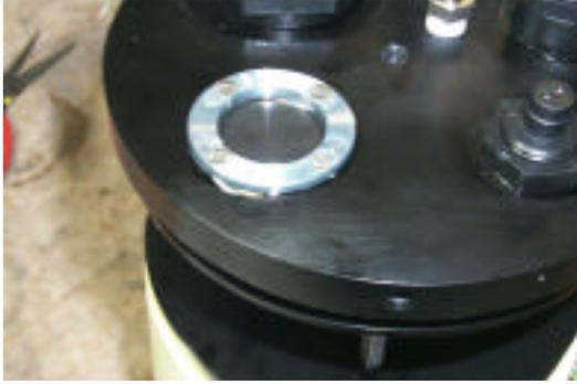
Remove the retaining ring and the neoprene membrane and set aside on a paper towel.
