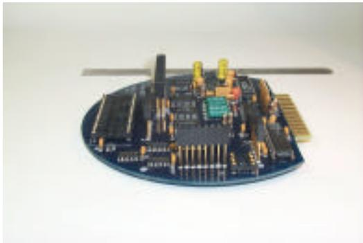
This view of the CPU/IO card shows an empty 8-pin socket (on the edge close to the camera). This socket is for the MAX483 IC supplied with the TAPS spares kit. Install this IC to obtain RS-485 communications. The notch on the IC goes towards the inside of the PCB. Note that the CPU card is not installed in this view to make the socket easier to see; it is not usually necessary to remove the CPU card to change these IC's.
