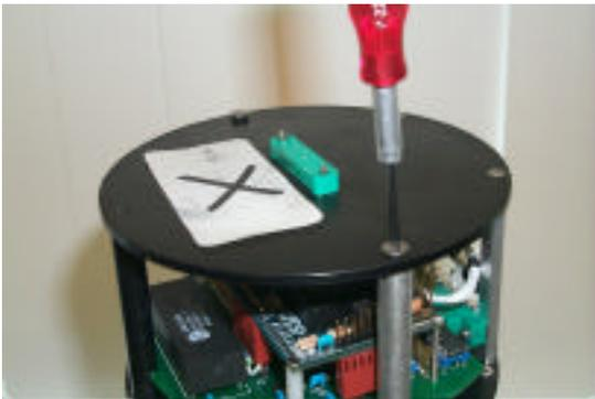
3. Remove the black delrin PCB (printed circuit board) retainer by lifting the top plate slightly (this is why you loosened the screws) and pulling the top of the rod out.
