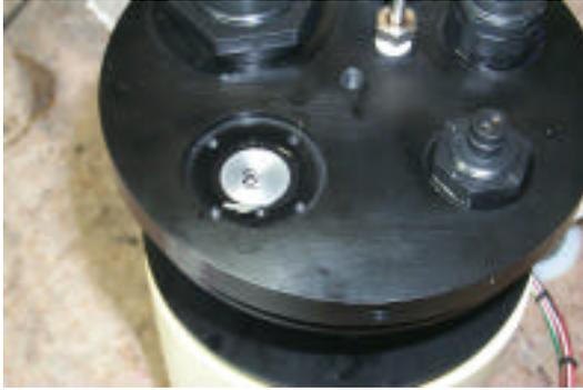
Place the neoprene cover gently in place, aligning the holes in the cover with the screw holes before dropping it into place. Lay the retaining ring in place over the cover. Install the four screws loosely, using a small dab of antiseize on each first. When all screws are installed,
