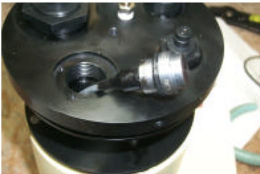
Prepare the new sensor for installation by installing an o-ring as shown below. Use a modest amount of
