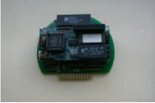
6. Install the new EPROM in this socket. One method for doing this is to place the IC over the socket and align the nearest row of pins with the mating jacks in the socket. Push these pins into the jacks slightly—just so they are located. Holding the IC at the ends, pull the entire IC back towards you while rotating the other row of pins towards the socket. When the pins appear to be aligned, push the IC firmly into the socket.
