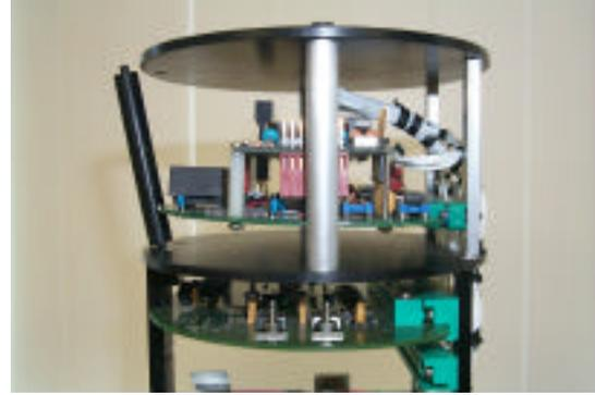
You may have to lift the rear edge of the PCB slightly to get the bottom peg out of it's hole.
